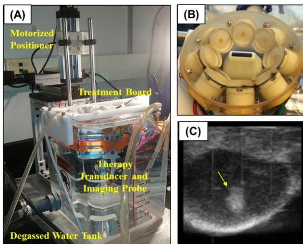
Figure 1. Experiment setup for therapy and imaging transducer mounted on the motorized positioning system and submerged in a tank of degassed water. (A) The animal is placed on the treatment board (B) 1 MHz therapeutic transducer with imaging probe coaxially mounted (C) Generation of echogenic bubble cloud in the target volume
