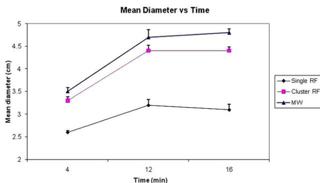
**Figure 1.** Graph shows the change in mean ablation diameter over time by the ablation device in an ex vivo bovine liver. MW ablations (triangles) are larger than single RF ablations (diamonds) at each time point. There was no statistical difference between MW ablations and cluster RF ablations (squares). Error bars represent standard error of the mean. (Available in color online at [www.jvir.org](http://www.jvir.org).)
