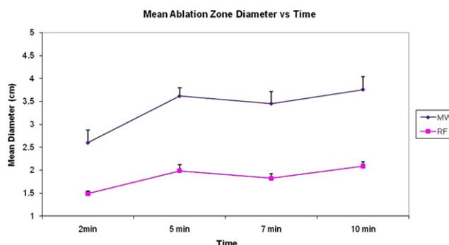
**Figure 3.** Graph shows mean diameter of the ablation zone over time by the ablation device in an in vivo porcine liver. As seen with the ex vivo data, MW ablations (diamonds) were significantly larger than RF ablations (squares) at all time points. Error bars represent standard error of the mean. (Available in color online at [www.jvir.org](http://www.jvir.org).)
