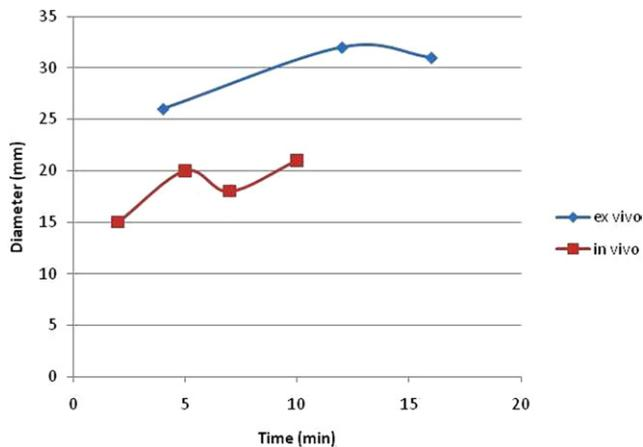
**Figure 6.** Graph comparing the ex vivo (bovine) and in vivo (porcine) mean RF ablation zone diameters over time. All ex vivo ablation zones are larger than the in vivo ablation zones, in contradistinction to the data seen for MW in **Figure 5**. (Available in color online at [www.jvir.org](http://www.jvir.org).)
